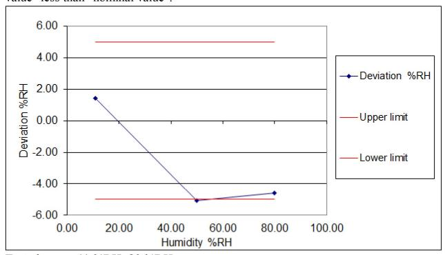
Tested range: 11 %RH÷80 %RH Measuring Instrument: 21-112,21-78
